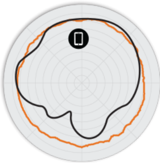
Figure 2. R500 2.4GHz Azimuth Antenna Patterns
