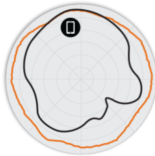
Figure 3. R600 5GHz Azimuth Antenna Patterns
