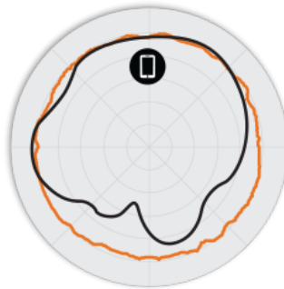
Figure 3. R500 5GHz Azimuth Antenna Patterns
