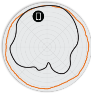
Figure 2. R600 2.4GHz Azimuth Antenna Patterns
